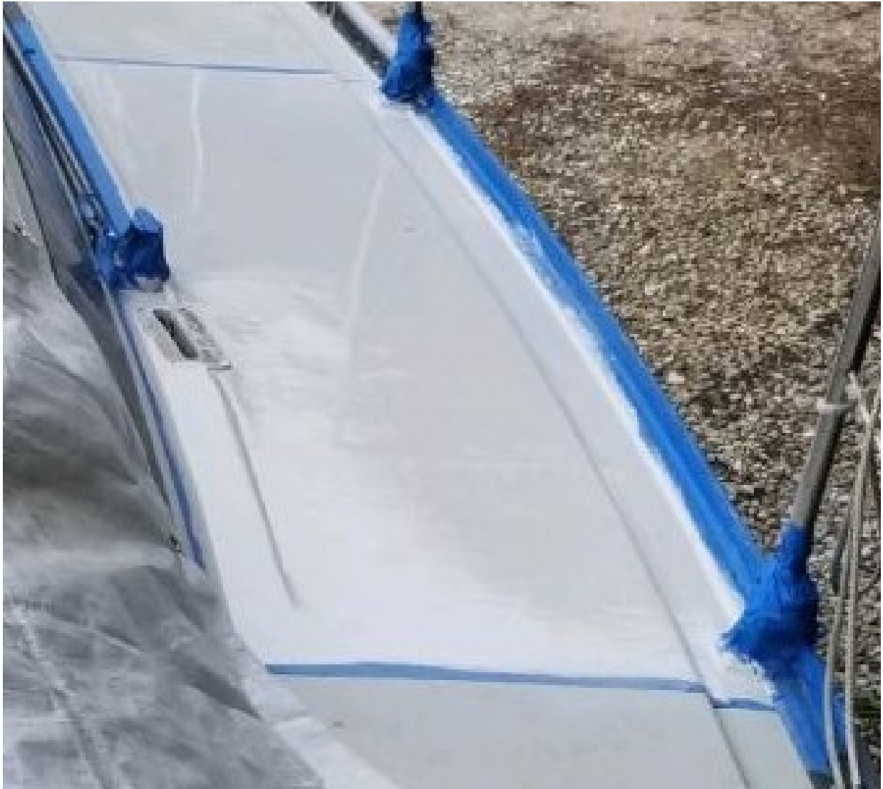
Port side; looking from bow; faired, sanded, primed and painted
