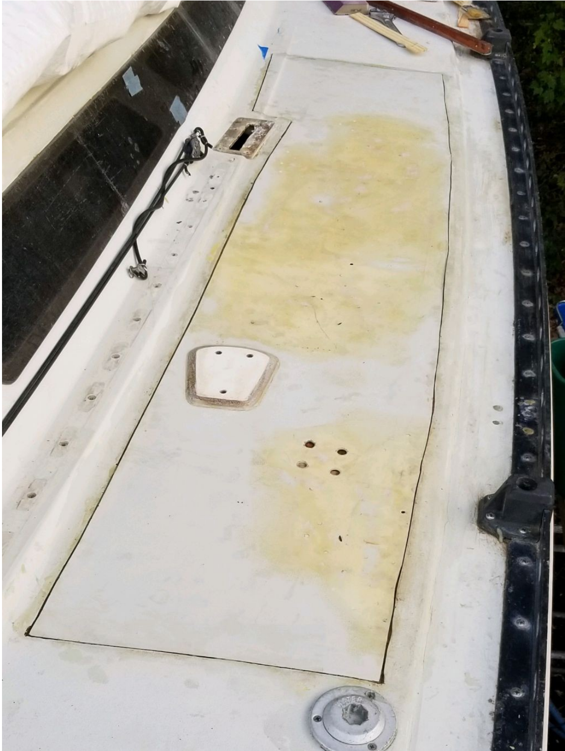
Starboard side; top skin back on
