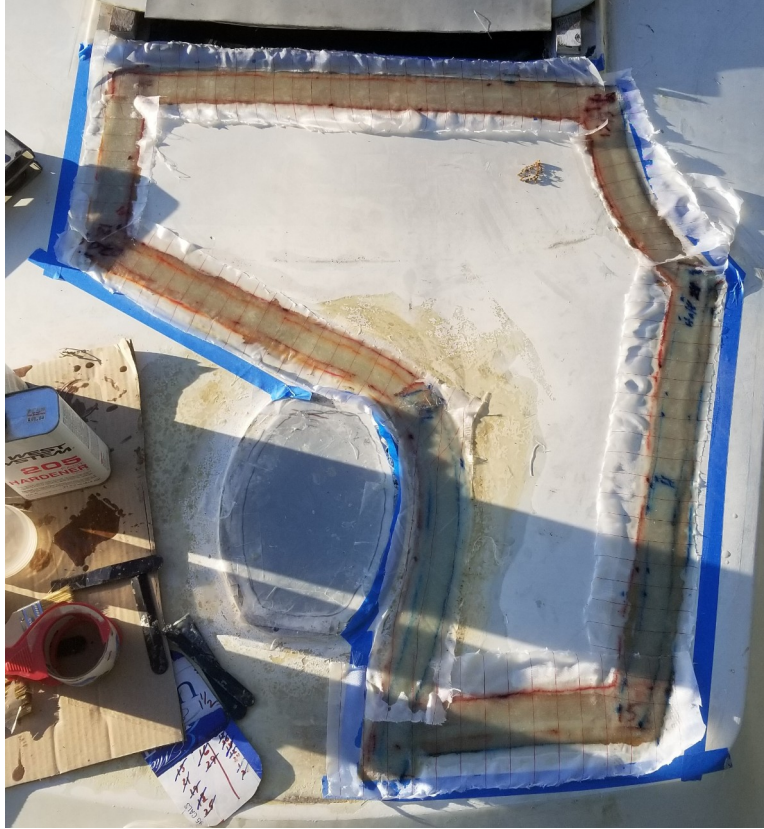
5) Strips of 1708 applied to the joint & covered in peeply.
