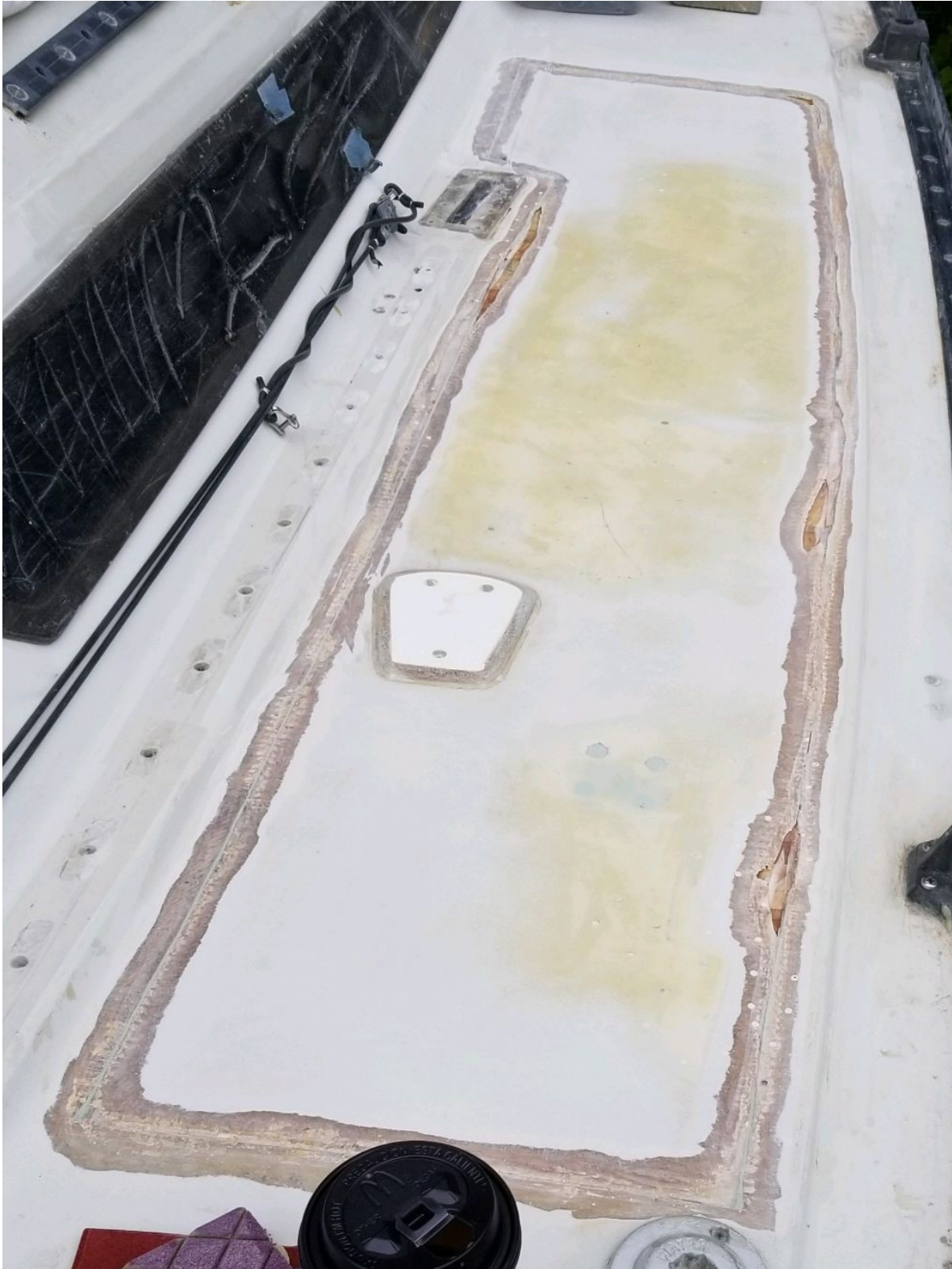
Starboard side; 12:1 bevel ground around the joint
