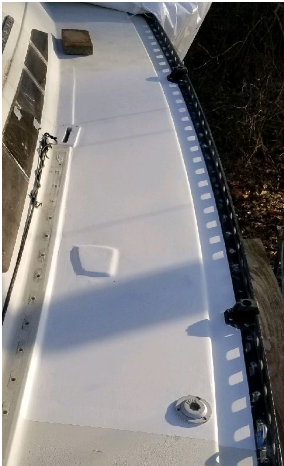
Starboard side; after a coat of primer, more fairing and a 2 nd coat of primer
