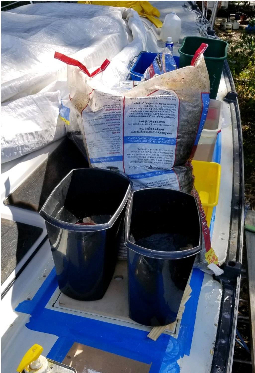
Starboard side; Top skin being epoxied back on, weighted with bags of birdseed and buckets of water placed on plywood scraps to spread the load. Sticks helped shim the edge flush with the deck
