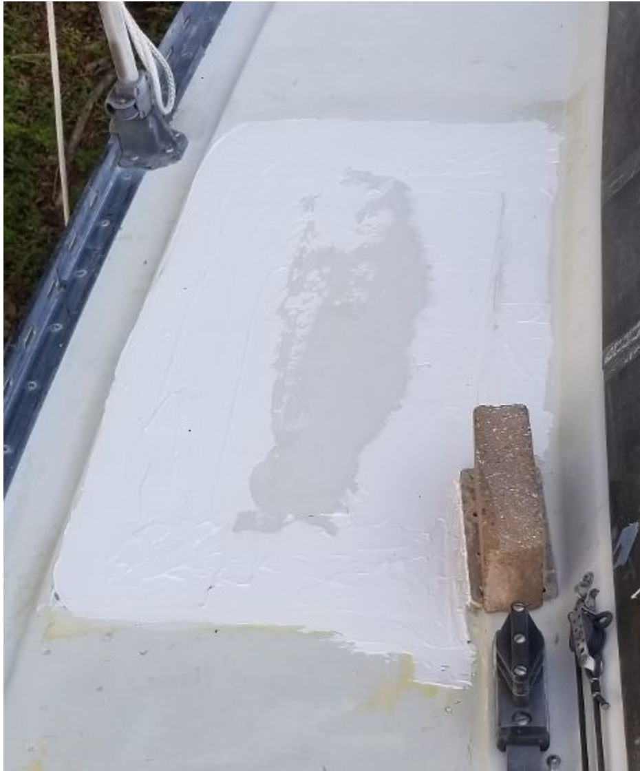
Port side; Area faired using Pettit EZ-Fair which is white. Photo taken before sanding.
