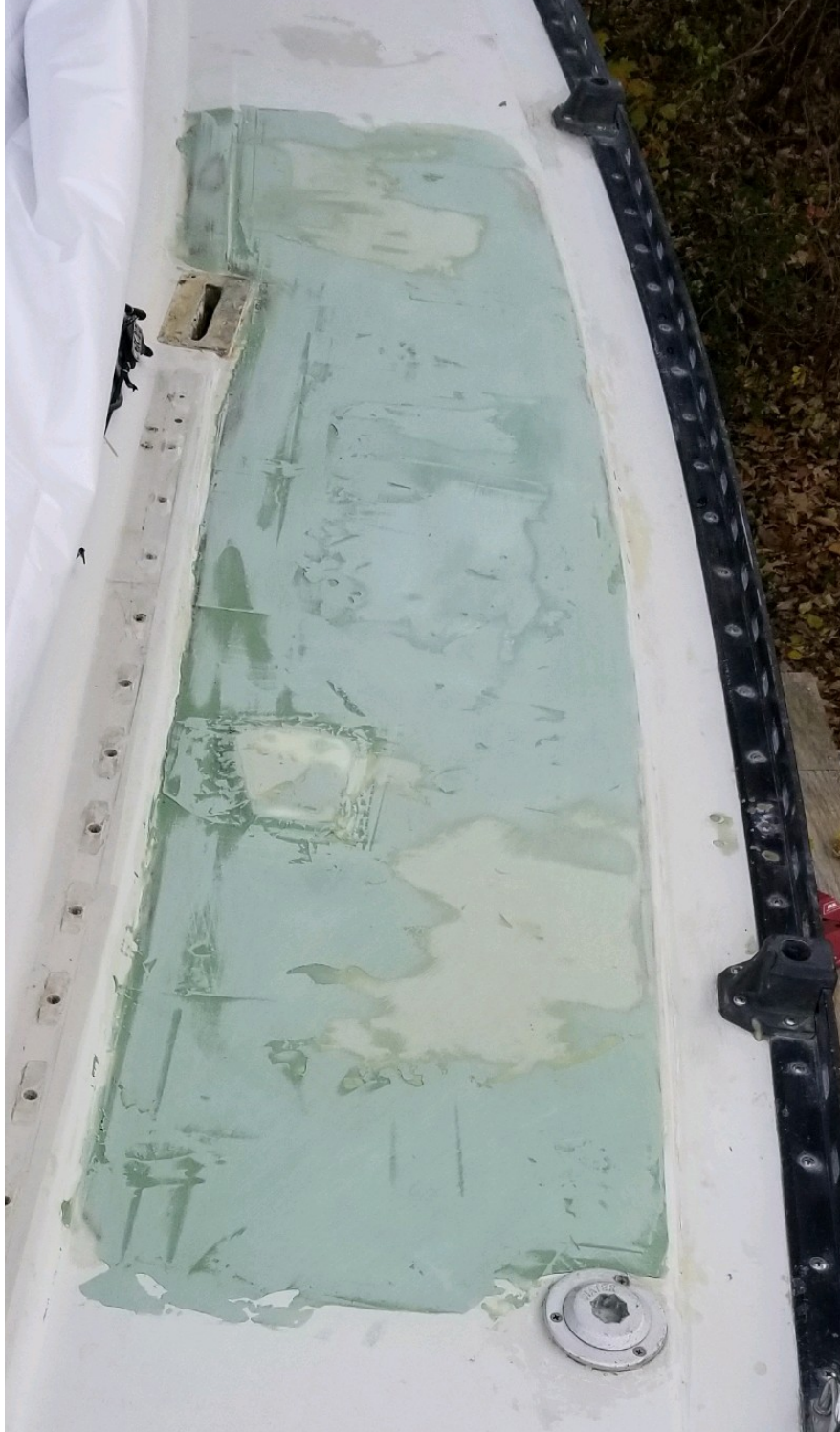
Starboard side; after several cycles of fairing and longboard sanding
