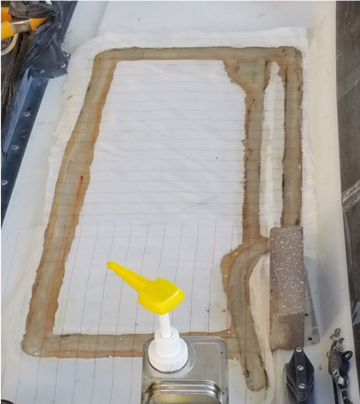
Port side; joint bevel filled with two layers of 1708 and covered with peelply
